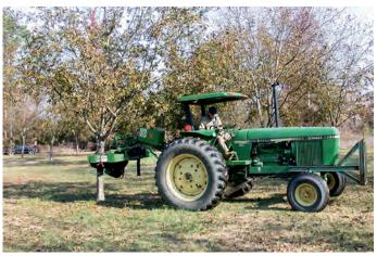
Figure 34. Shakers for removing nuts from the tree when mature are available in many different sizes for various sized trees and orchards.
