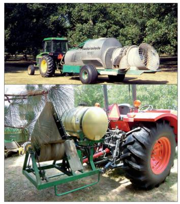
Figure 30. Air-blast orchard sprayers are most effective at managing insect and disease pressure and are available from various manufacturers in many different models and sizes.
