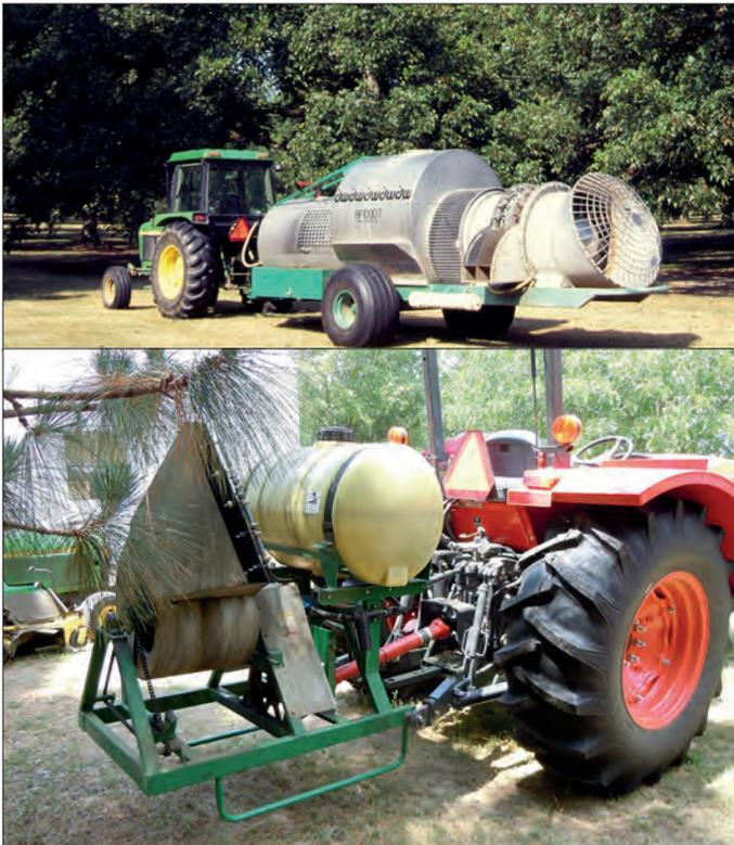
Figure 30. Air-blast orchard sprayers are most effective at managing insect and disease pressure and are available from various manufacturers in many different models and sizes.
