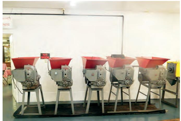
Figure 36. Pecan cracking devices crack the shells, which must be separated from the nuts.
