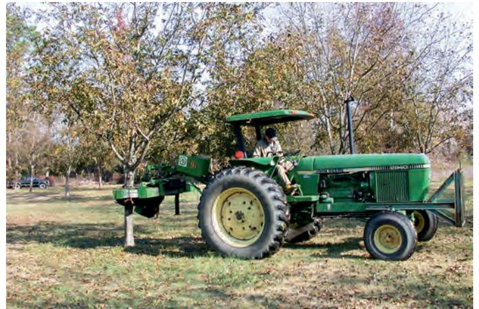
Figure 34. Shakers for removing nuts from the tree when mature are available in many different sizes for various sized trees and orchards.
